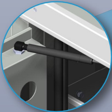
Door held open with gas struts
