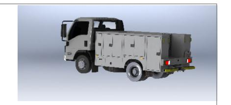
Volume: 2.5 cubic meter Body Weight: 800 kg
